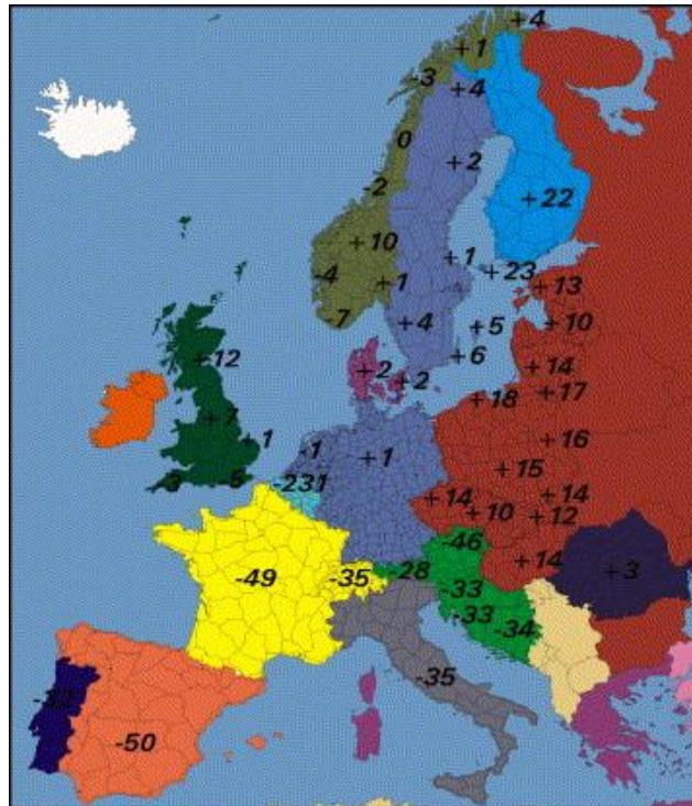
Figure 1. Transformation parameters from national heights to UELN height in Europe (values in cm).
